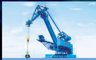
Level Luffing Crane
