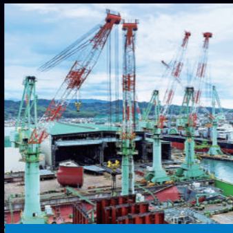
Rail Mounted Jib Crane
