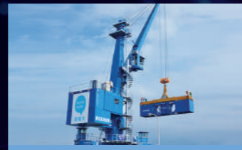
Tire Mounted Jib Crane
