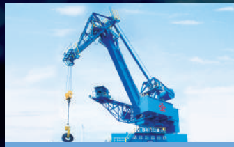
Level Luffing Crane
